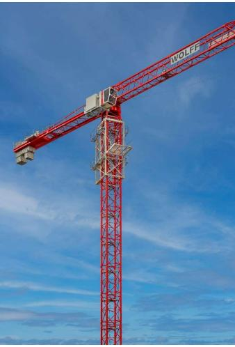
The jib design has been continuously refined over the years. The **WOLFF 8038** Clear features not only the functional new upper chord connection with a plug-in system but also a simplified lower chord construction, which uses less material and therefore reduces assembly weight.
