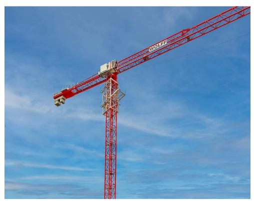
The WOLFF 8038 Clear combines the performance of a towertop crane with the assembly advantages of a flat-top design. It is shown here on the test site with an external climbing system for climbing tests.
