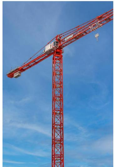
The WOLFF 8095 Compact is Wolffkran's largest trolley jib crane to date. It enters the 900-mt class with a reduced tower top section. As a result, it excels in both lifting capacity and assembly efficiency.
