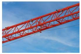
By designing the first three jib parts as a four-chord instead of a three-chord version, significantly higher lifting capacities are enabled. The hoist rope support on the jib reduces rope sag from seven to just 1.5 meters, making multi-crane operations safer.
