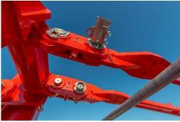
Assembly is further simplified by the supports for counter jib installation (I.) and the bolt storage (o.).
